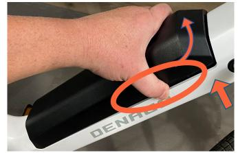
STEP 2-Grab battery with hand on indentation and lift back away from bike and UP and out of chamber holding battery
