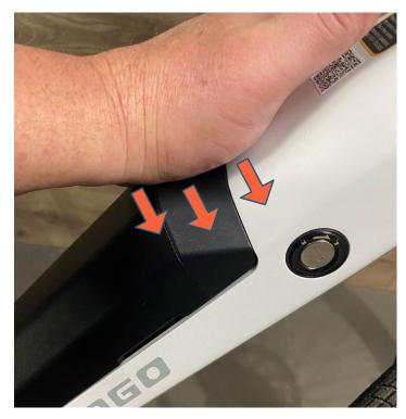
STEP 3 – Engage Battery Press firmly at top of battery until a CLICK/ENGAGMEMNT is heard
