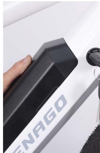
Return Battery Press Battery at TOP until you hear click
