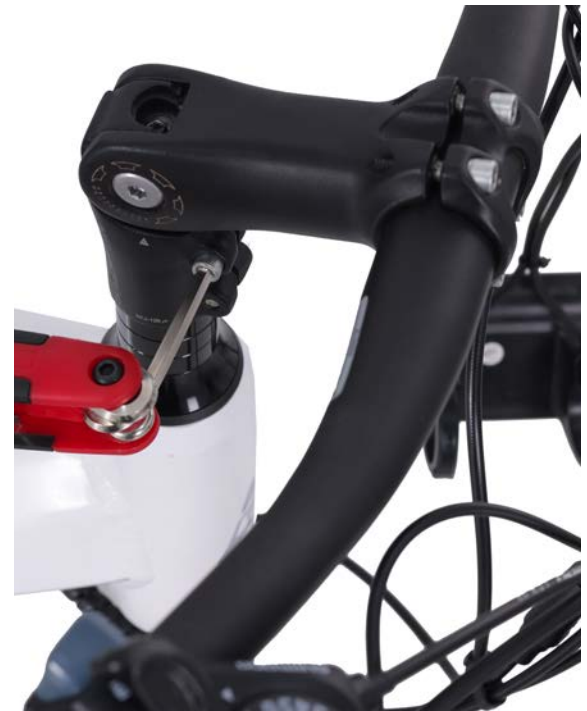
3. Place stem onto the head tube. Align stem to the center position.
