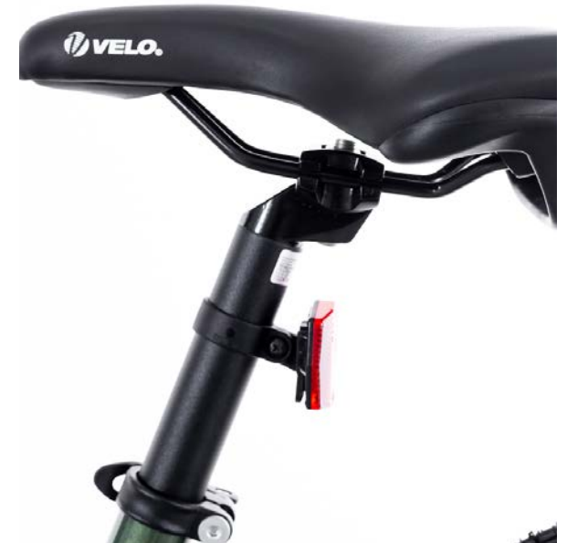
3. Place Seat Post inside Seat Tube - Insert past MIN Insertion Marking
