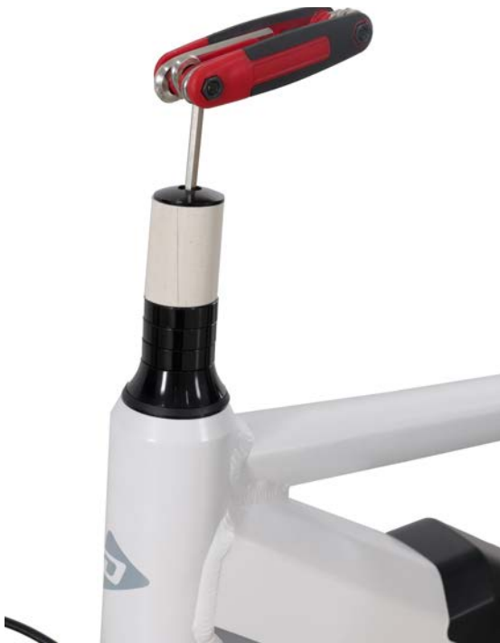
1. Unscrew bolt and remove cap, bolt, and sleeve. Leave all spacers in place.
