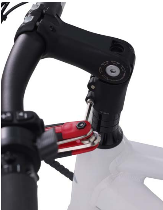
4. Tighten and Secure bolts on bottom of stem
