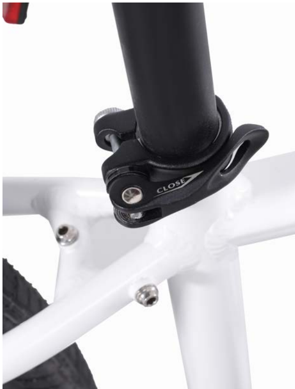
4. Adjust the seat height. Clamp secure/tighten the quick release clamp
