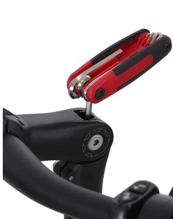
2. Place stem on steerer tube and tighten the bolt on top of stem to secure stem to front of bike
