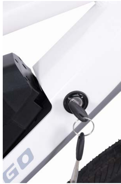
Lift Battery Out Be careful. It is heavy
