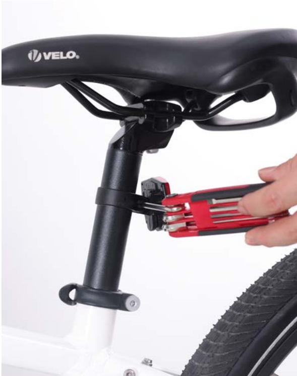
1. Install Rear Reflector (Red) to Seat Post
