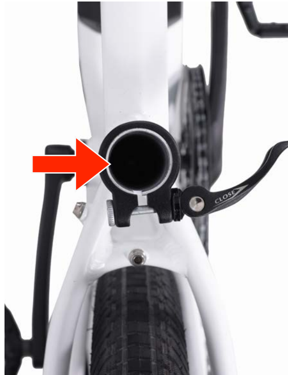
2. Apply grease inside Seat Tube
