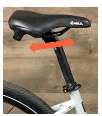
Step 3- Slide to proper position make sure seat is at proper angle (see Step 4) and then tighten bolt
