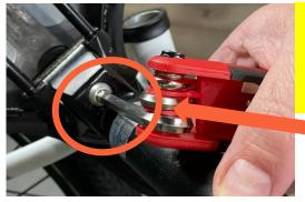
CAUTION- Ensure bolt is tight and secure. Otherwise, your saddle could rock, and bolt will break causing damage and injury
