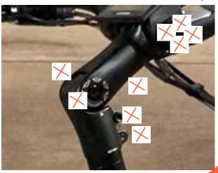
CAUTION- The Handlebar stem has 9 bolts that need to be properly secure and tighten to be safe. Failure to do so could cause serious injury or damage. If you are unsure or need help, please reach out to us at BIKE.com or your local bicycle shop prior to riding.
