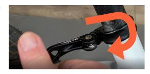
Step 3- Slide post UP or DOWN to meet proper alignment
