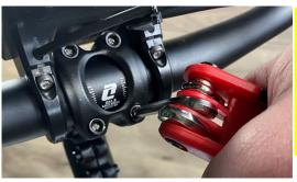
CAUTION- The Handlebar stem has 9 bolts that need to be properly secure and tighten to be safe. Failure to do so could cause serious injury or damage. If you are unsure or need help, please reach out to us at BIKE.com or your local bicycle shop prior to riding.
