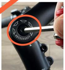
Step 3- Adjust the following bolt to loosen the stem to be able to adjust angle UP or DOWN
