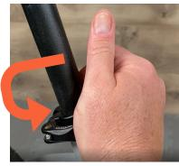
Step 4- Secure/CLOSE Quick Release Seat Binder. Try twisting seat to confirm secure. If not tighten adjust QR binder and secure.
