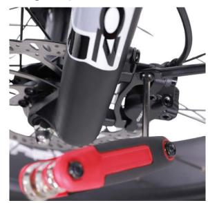
**2.** Align and secure fender support rods with included bolt into tapped area towards the bottom of the front fork.
