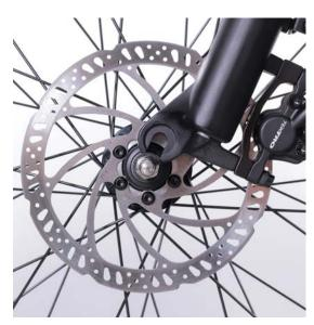
**2.** Position the front wheel so it's centered between the front fork legs with the axle resting inside the fork drop outs.
