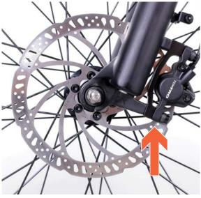
**3.** Align the disc brake rotor so it is centered in the slot of the brake caliper.
