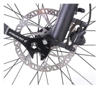
**4.** Tighten one axle nut part way then tighten the other nut, repeat until both sides are tightened securely. Be sure that the wheel is centered between the fork legs.
