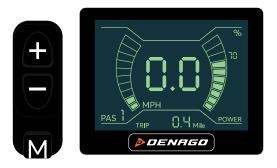
**STEP 1** – Press **M MODE** button until screen turns to either MAX speed or AVE speed.
