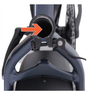
**2.** Apply grease inside Seat Tube.
