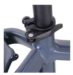
**4.** Adjust the seat height. Clamp secure/ tighten thequick release clamp.
