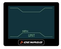
**SETTING 4 – unit:** This is the speed and distance setting MPH or KPH.
