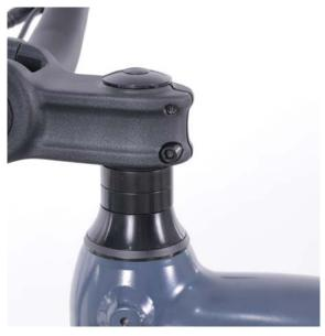
**6.** Upon final assembly, revisit this step to confirm alignment with stem and front wheel.
