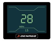
STEP 4 – Limited Speed mode - **(LS)** this is where you can adjust MAX speed.
