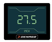
STEP 2 – Press + - (UP/Down) simultaneously for 2-4 seconds until screen flashes and goes to setting interface.
