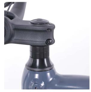
**4.** Tighten and secure ALL bolts on the stem. 7 positions to check and secure.
