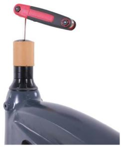
**1.** Using the 5mm allen key, unscrew bolt and remove cap, bolt, and sleeve. You will need the top cap and bolt in the next step. Leave all spacers in place.
