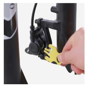
**1.** Remove Packing Block from disc brake caliper – Do Not Throw Away – Re-install Packing Block whenever you remove your front wheel.
