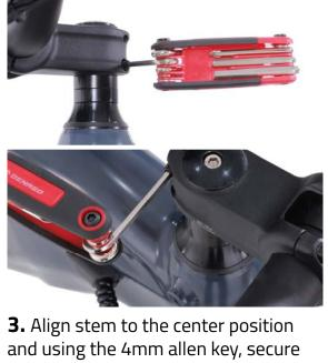
and tighten bolts on both sides of the stem.
