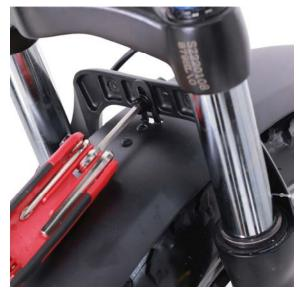
**1.** Locate Front Fork Brake Arch center hole and align front fender and insert bolt and nut thru brake arch and mounting bracket on fender. Secure and tighten.
