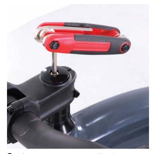
2. Place stem on steer tube & secure with bolt and top cap that was removed in STEP 1. Using the 5mm allen key, secure so no movement in headset area but it moves smoothly.
