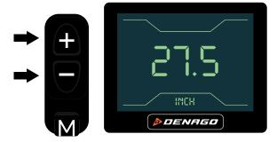
**STEP 2 – Press + - (UP/Down)** simultaneously for 2-4 seconds until screen flashes and goes to setting interface. You have 4 settings.
