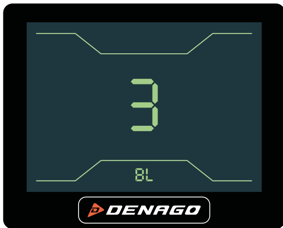
SETTING 3 – BL: this is screen brightness. You have 3 levels.
