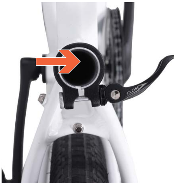
2. Apply grease inside Seat Tube
