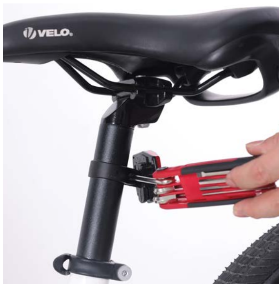
1. Install Rear Reflector (Red) to Seat Post
