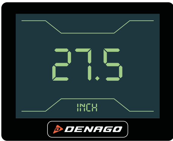
SETTING 1 - inCH: Wheel size setting. Your Denago City 1.0 is 27.5 .
